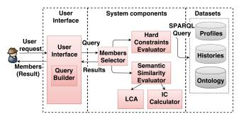
Figure 2: System Architecture
